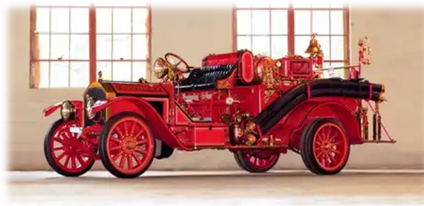
Fig 38. An example of the American-LaFrance auto triple combination pump used by the original Tucson Fire Dept #4 in Menlo Park. This model carried a 100-gallon tank and a pump that could empty the tank in 10 seconds. (Photo from wikipedia.org)
